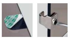
Decidethe pull position, stick the double-sided adhesive pad onto the glass door. Peel off the protective foil. Place the glass door, the side with the pad facing outwards, into the pull. Tighten the fixing screw. (max. 2 Nm).
